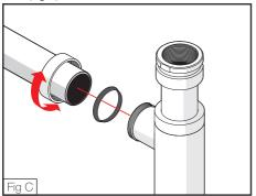
Lubricate the Kee seal and push-fit the Bottletrap and Outlet Pipe assembly into the elbow coupling. (Fig E)
