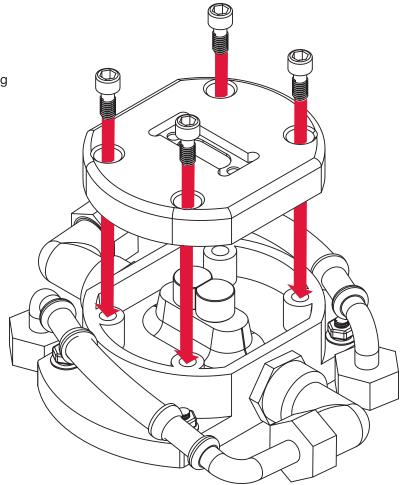
With the testing caps and brass cover still in place, turn on the mains water supply and test the connections for leaks. If any leaks are present, turn off mains water and check the seals on each of the hose connections.
