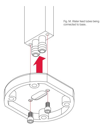
Push fit the outlet assembly onto the Mounting Base then use the 4 screws with spring washers supplied to fix the body down to the base with a 5mm Alley Key (provided).
