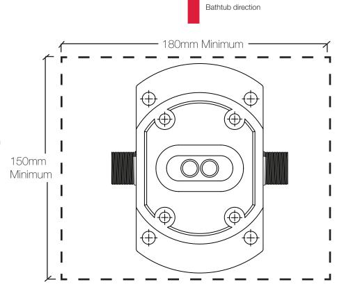
**Please note:** The depth of the floor pit will dictate the overall height of the Bath Filler once installed. The bottom plate of the Bath Filler body may sit on or underneath the tiled floor surface, but the base must remain underneath.
