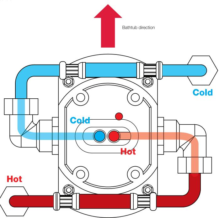
Fig. L. Layout of hot and cold water lines.
