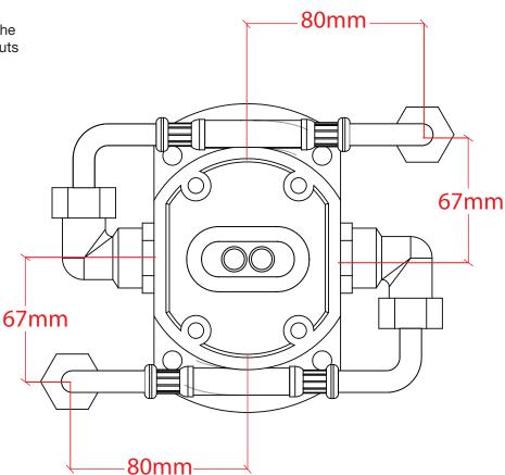
Fig. K. Water lines flexing to allow small shift of floor outlet location.
