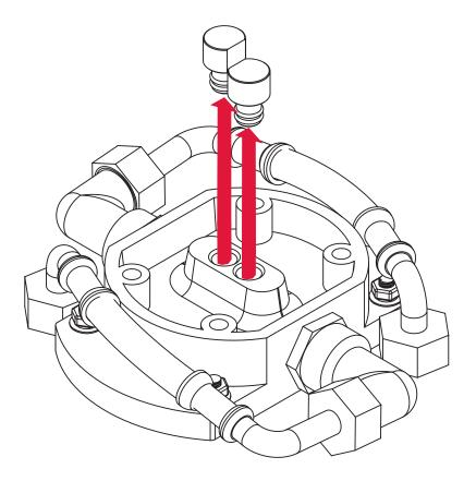
Fit the floor base cover over the Bath Filler outlet.
