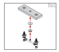
Allign the plastic washers below the outlet hole of the benchtop surface. Then insert the tee-piece (Fig B).
