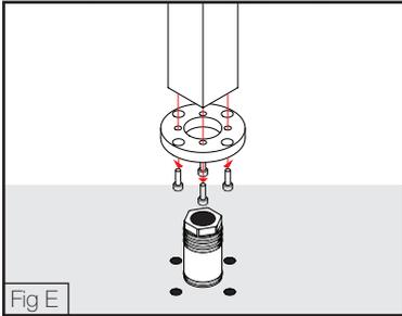
6. Slide the Chrome cover flange (2) onto the Spa outlet (1). (FIG F)
