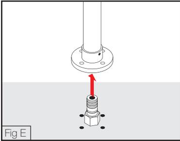
7. Slide the Chrome cover flange (2) onto the outlet (1) (FIG G)
