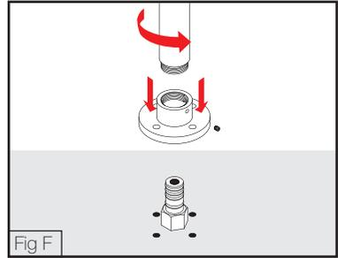
8. Screw Spa outlet (1) onto Brass base (3), then tighten grub screw with 2mm Allen Key (FIG H)
