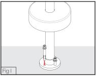
Align spa outlet to desired position, then mark holes on floor surface. (FIG D)
