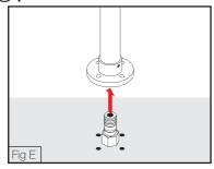
Slide the Chrome cover flange (2) onto the outlet (1) (FIG G)
