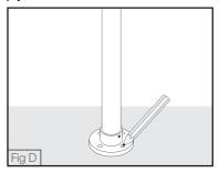
Unscrew and remove Brass base (3) from the Spa outlet (1). (FIG F)
