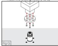
Use the optional Dyna-bolts to mount Spa outlet (1) to floor. (FIG I)
