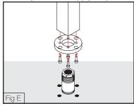
Secure the Brass cover plate (3) back under the Spa outlet (1) making sure to match the existing holes. (FIG G)
