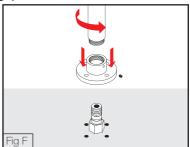
Screw Spa outlet (1) onto Bass base (3), then tighten grub screw with 2mm Allen Key (FIG H)
