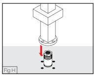
Slide Chrome cover flange (2) to floor surface to complete installation. (FIG J)
