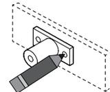
3. Drill the mounting holes to suit the plastic plugs provided
