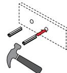
5. Install screws through the plastic plugs into the wall, where appropriate, fit locking rings or collars over the plastic plugs before installing screws. Install and tighten any grub screws supplied.
