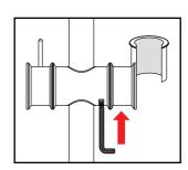
3. Retighten the grub screw until firm fit
