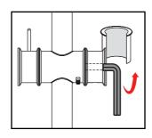
2. Tighten the screw inisde the slider
