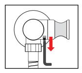
Loosen the grub screw inside the slider with an Allen Key
