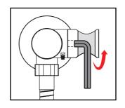
2. Tighten the screw inisde the slider
