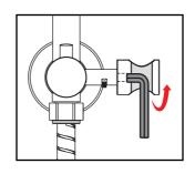
2. Tighten the screw inisde the slider
