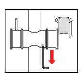
1. Loosen the grub screw inside the slider with an Allen Key
