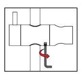
1. Retighten the grub screw inside the slider
