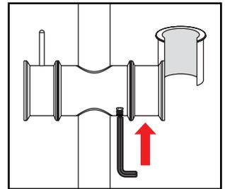
3. Retighten the grub screw until firm fit
