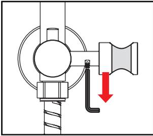
1. Loosen the grub screw inside the slider with an Allen Key
