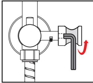
2. Tighten the screw inside the slider
