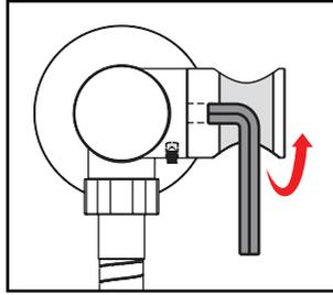
2. Tighten the screw inside the slider
