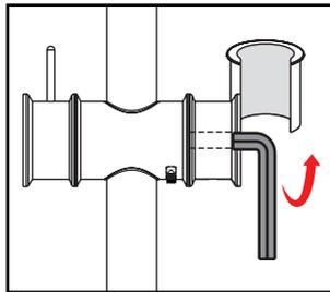
2. Tighten the screw inside the slider
