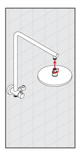
Attach the Hose (5) to the Handpiece (4) the tighten to the base of the Divertor Body (3).
