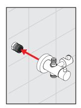
Push fit the Shower Arm (1) onto the nipple of the Divertor Body (3). Tighten the grub screw to secure the arm to the nipple.
