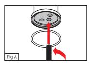
Apply lubricant to the o-rings of the Water Hoses (2). Then insert and tighten them underneath the Basin Mixer Body (1) to the matching colour indicators [Fig B]
