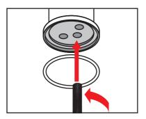
Allign and place the assembled body (1) and hoses (2) into the basin mounting hole.
