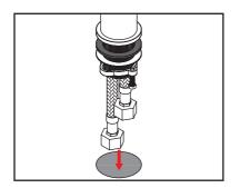
From the underside, fit the washers and locknut ring over the brass sleeve (4). Use the bolted locknut (5) to screw in and tighten in place
