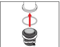
Apply lubricant to the orthogon. Then insert and tighten them underneath the Basin Mixer Body (1) to the matching colour indicators.
