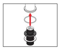
Allign and place the assembled body (1) and hoses (2) into the basin mounting hole.
