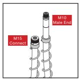
Insert the new hose with the M10 male end connection carefully through the body past the outlet end as shown
