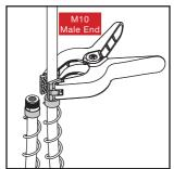
Unscrew the nut that connects to the mixer in anti-clockwise direction. At all times ensure plastic stopper is on the end of both sides of the spring
