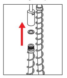
Apply lubricant to the o-rings of the Water Hoses (2). Then insert and tighten them underneath the Sink Mixer Body (1) to the matching colour indicators.
