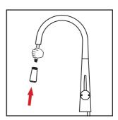
Remove clamp and slowly retract spring coil back up along the hose. You have now successfully reassembled the hose
