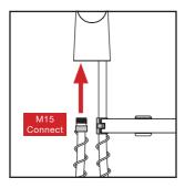
Retract the spring coil to remove tension. Insert a clamp to hold the hose and ease the installation
