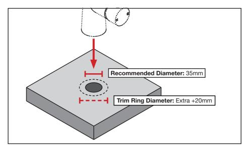
Ensure the cutout for the Hob Pull-Out Sink Mixer is 35mm in diameter
