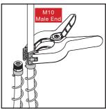
Hold the hose and install nozzle enusuring a tight fitment
