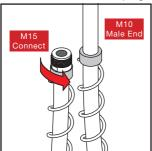
Unscrew the pull out nozzle and push into outlet
