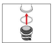
Apply lubricant to the o-rings of the Water Hoses (2). Then insert and tighten them underneath the Sink Mixer Body (1) to the matching colour indicators.
