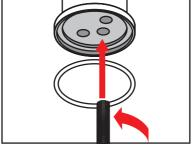
Apply lubricant to the ornings of the Hoses (2). Then insert and tighten them underneath the Sink Mixer Body (1) to the Apply lubricant to the o-rings of the Water matching colour indicators.
