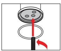
Apply lubricant to the o-rings of the Water Hoses (2). Then insert and tighten them underneath the Sink Mixer Body (1) to the matching colour indicators.
