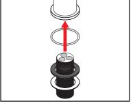
Apply lubricant to the ornings of the Hoses (2). Then insert and tighten them underneath the Sink Mixer Body (1) to the Apply lubricant to the o-rings of the Water matching colour indicators.
