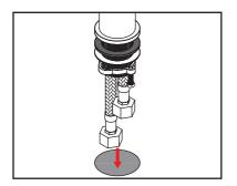
From the underside, fit the washers and locknut ring over the brass mount (4).
