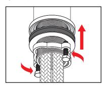
After installation, ensure that the mixer is secured firmly and there are no signs of any leaks
