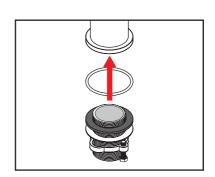
Apply lubricant to the o-rings of the Water Hoses (2). Then insert and tighten them underneath the Sink Mixer Body (1) to the matching colour indicators.
