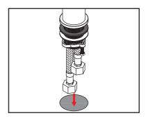
From the underside, fit the washers and locknut ring over the brass mount (4). Use the bolted locknut (5) to screw in and tighten in place
