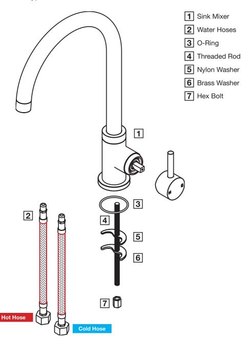
Insert and screw the Brass Thread Rod (4) underneath the Sink Mixer Body (1) and place the O-Ring (3) under the base plate
