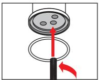
Allign and place the assembled body (1) and hoses (2) into the sink mounting hole.
