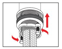
Insert the O-Ring (1) under the base plate. Then screw in the Brass Mount (4) under the Basin Sink Body (1)
