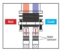
5. From the underside, fit the washers and locknut ring over the brass mount (4). Use the bolted locknut (5) to screw in and tighten in place
