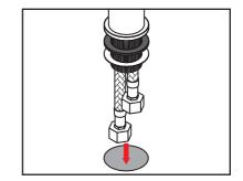
After installation, ensure that the mixer is secured firmly and there are no signs of any leaks
