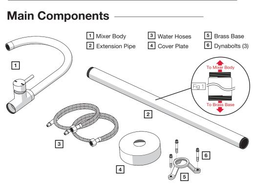
Please Note: Extension Pipe thread differ at each end. Please ensure that extension pipe in in the correct orientation before following installation steps. Please Refer to Fig 1.
