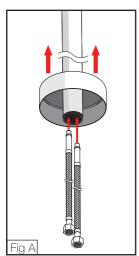
2 Apply lubricant to the Flexible water Hoses (3) O-rings, and install into the underside of the Mixer Body (1). (Fig B)
