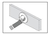
Tap the Wall Plugs into place and ready to insert the Wall Brackets
