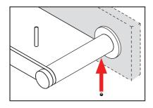
Drill the mounting holes to suit the plastic Wall Plugs
