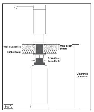
Prior to installing, calculate the finished benchtop thickness to ensure the Flange and Soap Pump Assembly will fit the final assembly.
