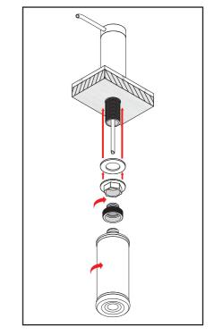
$\sum$  . Slide the rubber washer up on the timber deck. Then secure the washer with the screw lock.
