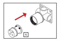
Re-Insert the Mixer Cartridge in correct orientation using the location pins.
