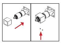
Insert the Brass Body Extension (1) into the Mixer Body. Ensure that the location pins are orientated correctly within the body.
