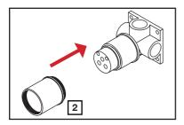
Slide Mixer Body Sleeve over the Extension Sleeve (2). Tighten grub screws to secure.
