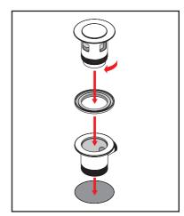
Slide the Operting Rod (5) on the Waste Base (3). Then fit in the Ball Joint Parts (4) and tighten firmly to close it. Insert the Control Extender (8) to the L Shpared Connector (7). Then screw in and connect to the Control Rod (6) to enable the pop-up action
