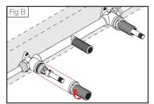
Install the outlet (8) prior to the domes (6) to secure the backplate (5) to wall surface. Please ensue that the backplate is level before tightening.
