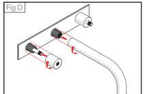
Slide the Backplate (5) over the ceramic disc assembly (3) onto the finished wall.
