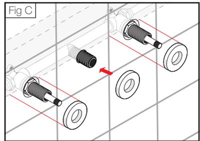
5. Install the outlet (8) prior to the domes (6) to secure the backplate (5) to wall surface. Please ensure that the backplate is level before tightening.
