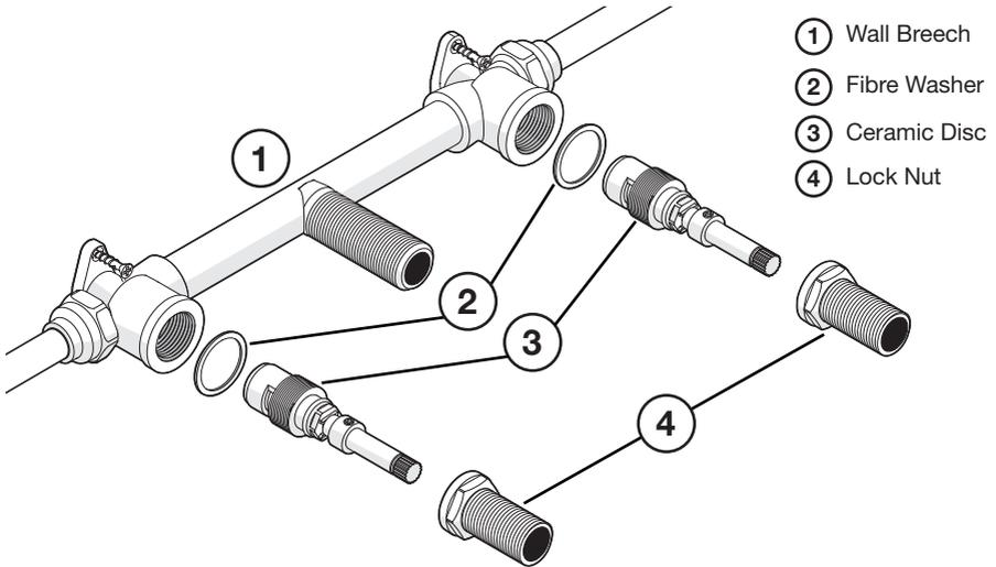
1. Prior to installing ceramic disc assembly make sure the seat surface is clean and smooth otherwise reseal and recheck. Also ensure that lines have been flushed.
