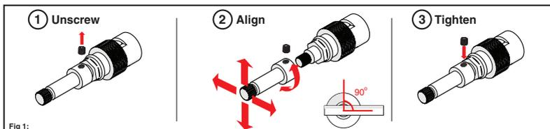
Firstly ensure that the disc is in the closed position and then fit handle to align.
