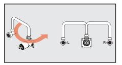
**Note:** Please ensure that the noggin depth behind the face of the wall is within specification, (40mm to 70mm from Finished Wall, See Left Drawing)
