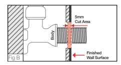
Fit the 1/2 Inch Outlet Thread (6) into the Wall Breech (7). Ensure a thread sealer has been applied and tighten with a 12mm Allen Key.
