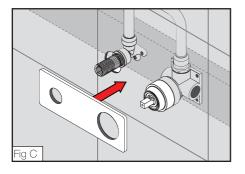
Fit the 1/2 Inch Outlet Thread (4) into the Wall Breech (6). Ensure a thread sealer has been applied and tighten with a 12mm Allen Key.
